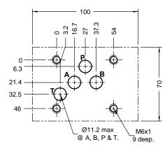
**Note:** Valve fixing S.H.C Screws are not in scope of supply. Tightening torque for S.H.C Screws is 16 Nm.
